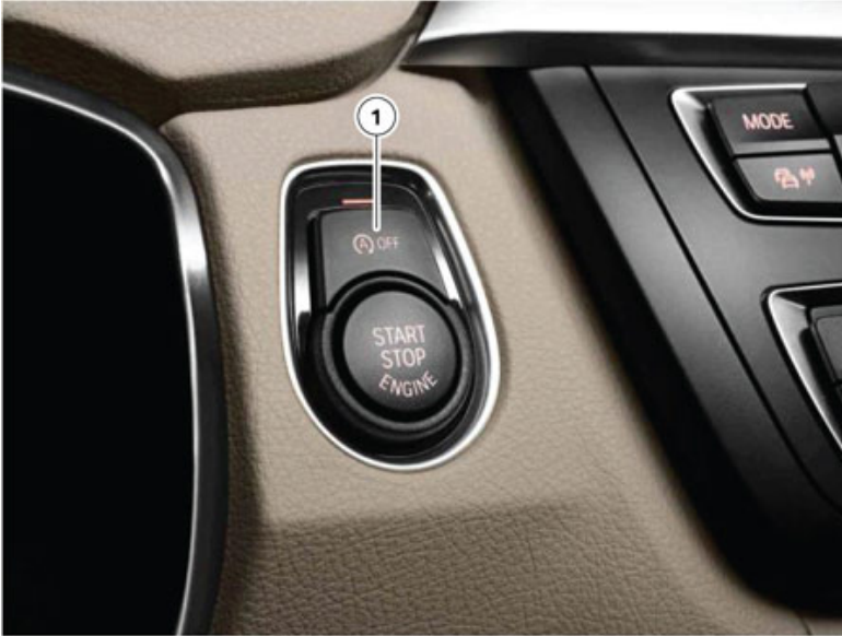
F30 automatic start/stop function button location
